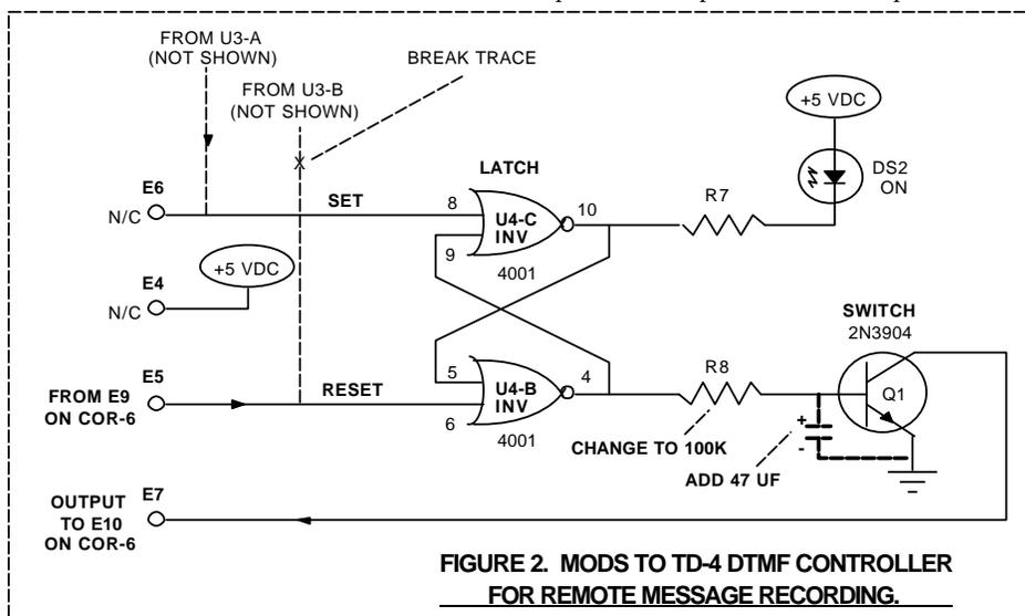
board from U3-B to U4-B as shown. Then, change R8 on the TD-4 to 100K, and add a 47µF electrolytic capacitor from the base of Q1 to ground, as shown.
