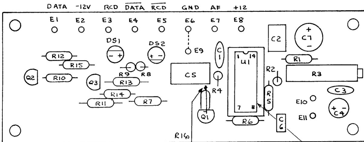
Note: Some of the LEDs have their positive lead on the right side and others have a longer positive lead than negative.
