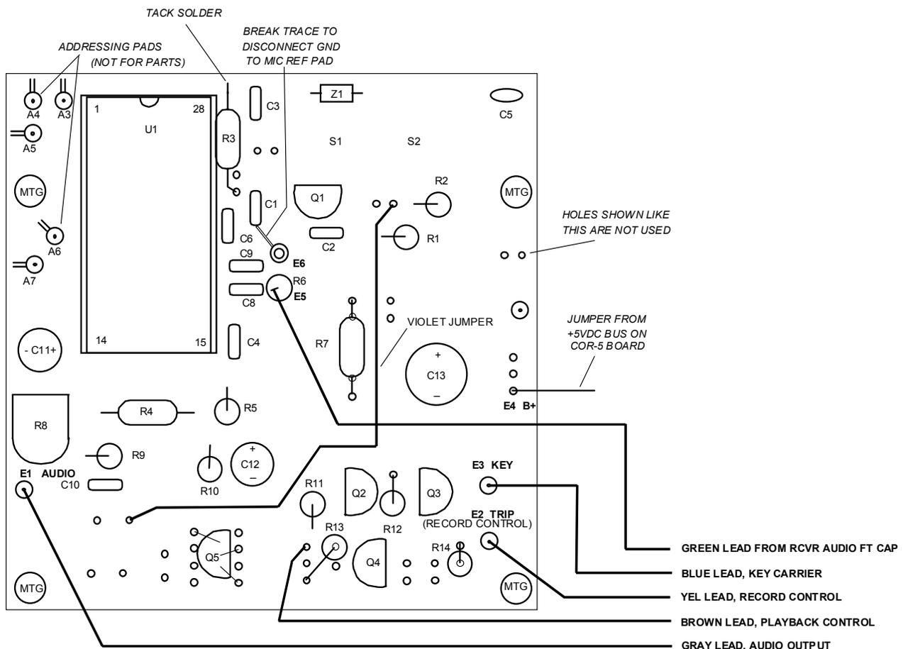
Note: Q6 and R15 are located under board and are not shown here.
