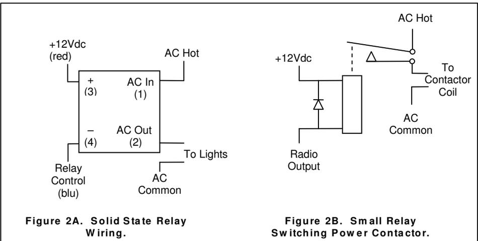
Figure 2A. Solid State Relay Wiring.
