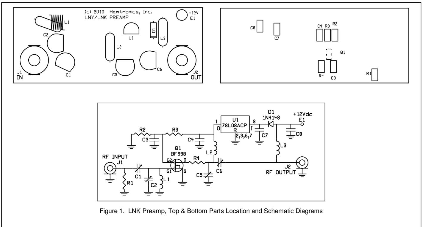
Figure 1. LNK Preamp, Top & Bottom Parts Location and Schematic Diagrams
