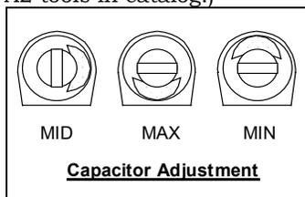
All variable capacitors should be preset to the center of their range unless the unit has been previously
