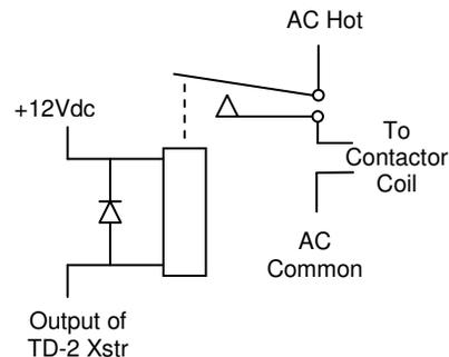
**Figure 3B. Small Relay Switching Power Contactor.**
